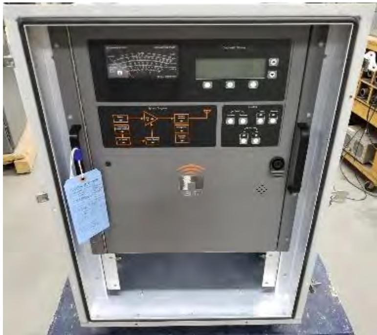
VR125 Installed in IP66 rated Cabinet
