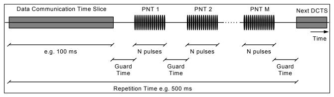
Figure C1: Time sequence of a possible LF PNT&D system
