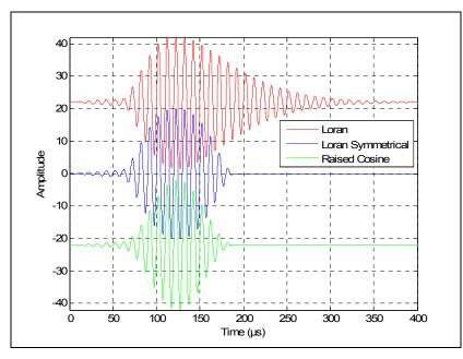
Figure C5: Simulated, received, and composite pulses with 26 dB stronger skywave
