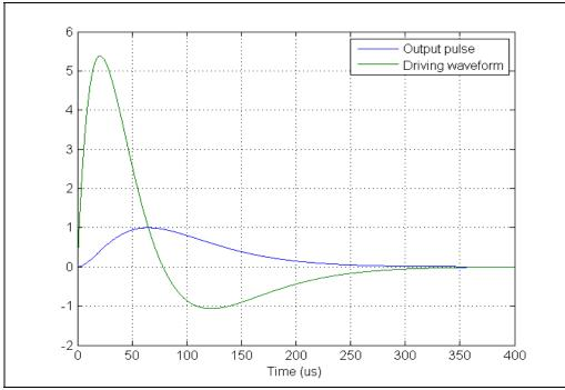
Figure B4: Desired Loran pulse along with the driving waveform required to achieve it into an antenna system with a Q of 60
