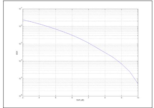
Figure B2: Uncoded bit error rate vs. received SNR for the proposed signal
