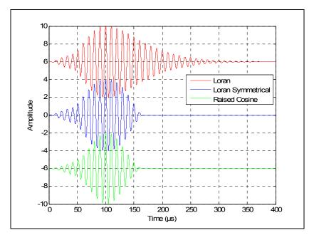
Figure C4: Simulated, received, and composite pulses with 12 dB stronger skywave
